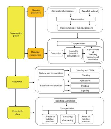
Figure 6: Suggested Framework of ECE-LCA Tool: All LCA Stages
